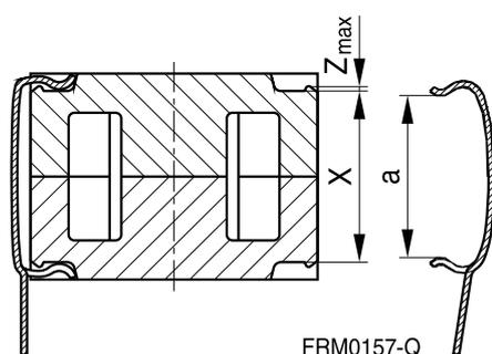
$F_{min}$ : Extension of clamp from  $a$  to  $a_2 = X_{min}$
