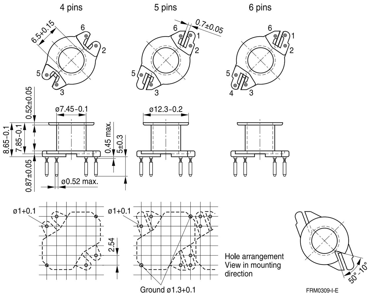
**Coil former for SMPS transformers with line isolation**
