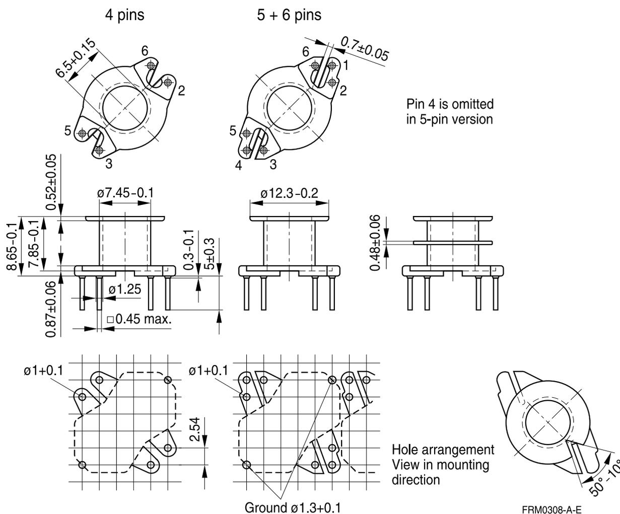
**Coil former, pins squared in the start-of-winding area**
