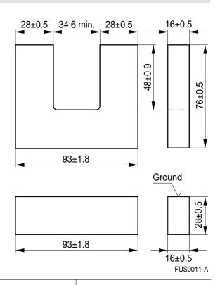
The  $A_L$  value in the table applies to a core set comprising two ungapped cores.
