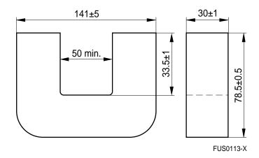
The  $A_L$  value in the table applies to a core set comprising two ungapped cores.
