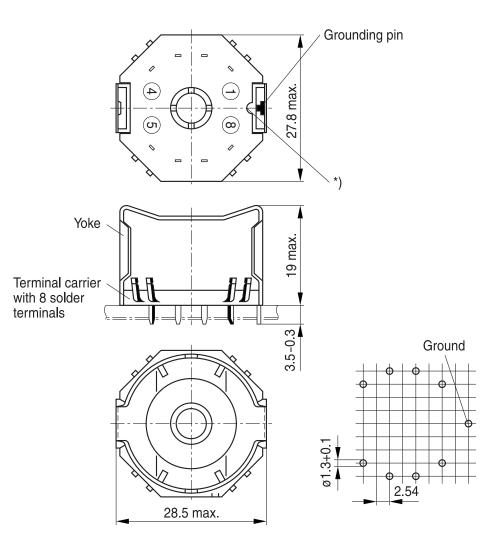
\*) This recess must be on the side of the grounding pin to ensure that the yoke locks into position.
