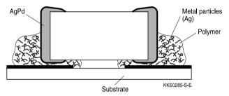
Attaching surface-mounted devices (SMDs) with electrically conductive adhesives is a commercially attractive method of component connection to supplement or even replace conventional soldering methods.
