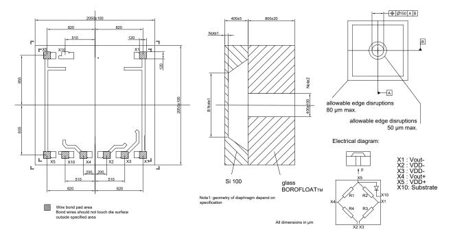
All technical data are defined for pressure application from passive side. Sign of output voltage will change by pressure application from active side.
