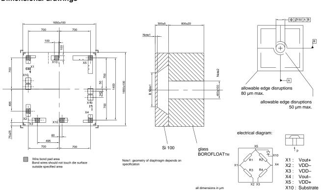
All technical data are defined for pressure application from passive side. Sign of output voltage will change by pressure application from active side.
