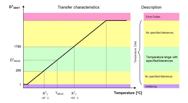
Conversation SENT's Temperature Data to physical Temperature acc. to conversation formula below.
