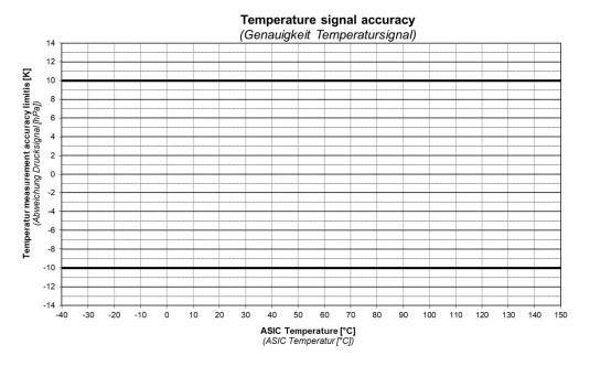
ASIC temperature measurement accuracy: +/- 10 K
