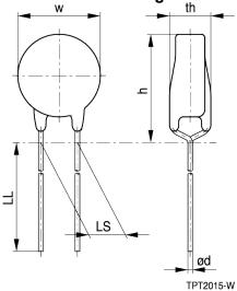
13.0 mm Wmax 5.0 th<sub>max</sub> mm 18.0 mm  $h_{\text{max}}$ d  $0.6 \pm 0.05$ mm LS 5.0 +0.6/-0.1 mm 25.0 LLmin mm
