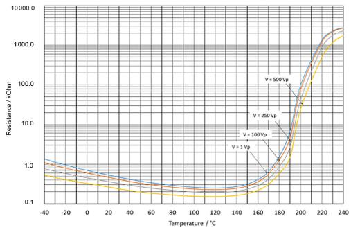
PTC resistance  $R_{\text{PTC}}$  versus PTC temperature  $T_{\text{PTC}}$
