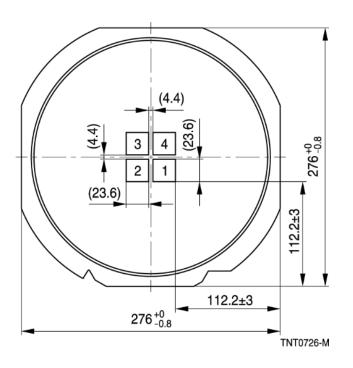
The 8" frame is loaded with chips, arranged in 1 to 4 arrays, beginning with array 1. Single chip positions can be empty because of removed parts for optical or electrical inspection.
