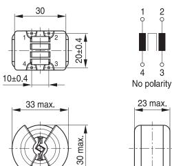
Part tolerances to ISO 2768-c / ISO 8015 Size ISO 14405 (E) All dimensions in mm
