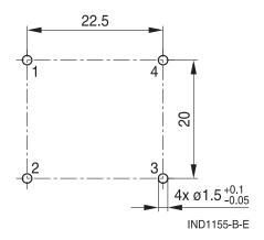
Part tolerances to ISO 2768-c / ISO 8015. Size ISO 14405 (E) All dimensions in mm
