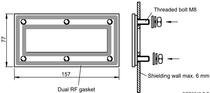
**Adapter flange for fixing holes**
