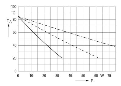
Permissible ambient temperature T<sub>A</sub> vs. total power dissipation P
