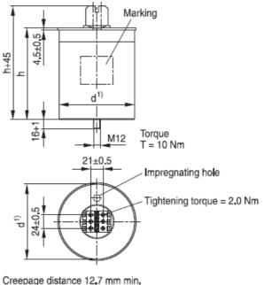
Creepage distance 12.7 mm n Clearance 9.6 mm min.
