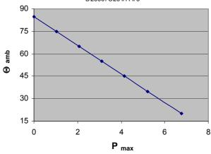
Max. allowable ambient Temp. at specific current (rms)
