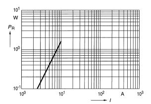
Ohmic power dissipation  $P_R$  versus rms current value I  $P_R$  (85 °C) = 16 m $\Omega$
