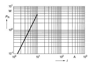
Ohmic power dissipation  $P_{\rm R}$  versus rms current value I  $R_{\rm S}$  (85 °C) = 48 m $\Omega$
