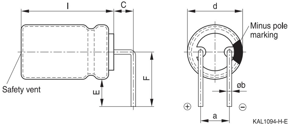
The series B41897, B41898 and B41899 have no sleeve nor minus pole marking, the positive pole is marked on the aluminum case side instead.
