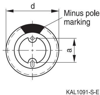
The series B41897, B41898 and B41899 have no sleeve nor minus pole marking, the positive pole is marked on the aluminum case side instead.
