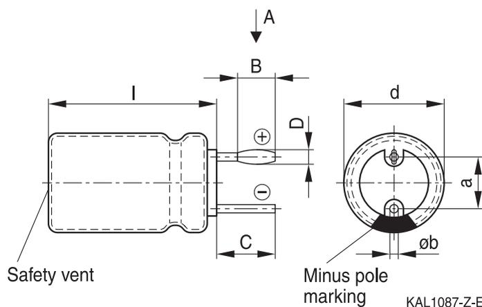
The series B41897, B41898 and B41899 have no sleeve nor minus pole marking, the positive pole is marked on the aluminum case side instead.
