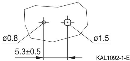
Suggestion for PCB hole diameter, wire  $\varnothing 0.8$  mm
