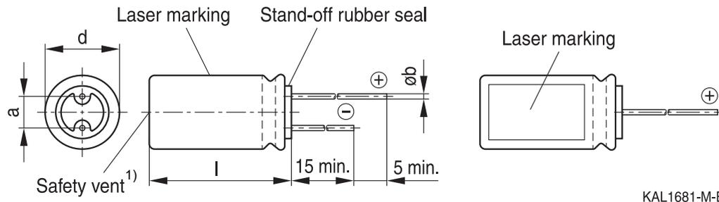
1) Supplied components may have different safety vent designs. They all offer the same safety vent functionality as pressure relief device.
