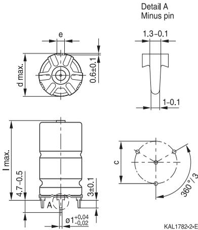
Mounting holes  $d = 21 \text{ mm}$
