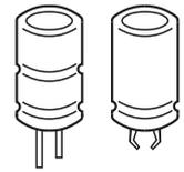
**Large-size capacitor, snap-in version high vibration stability (with middle corrugation)**
