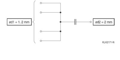
**Note**: 4 × 1.2 mm terminal-electrode (d1) 1 × 2 mm terminal-electrode (d2)
