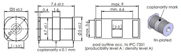
\* for reflow soldering, coplanarity mark upwards
