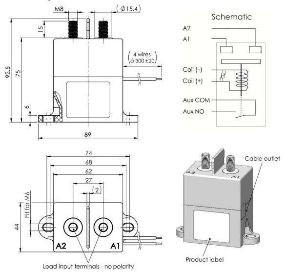
In case of no tolerance shown in dimensional drawing, general tolerances apply: dimension  $\leq$  10 mm: ± 0.3 mm; dimension 10 to 50 mm: ± 0.6 mm; dimension > 50 mm: ± 1 mm
