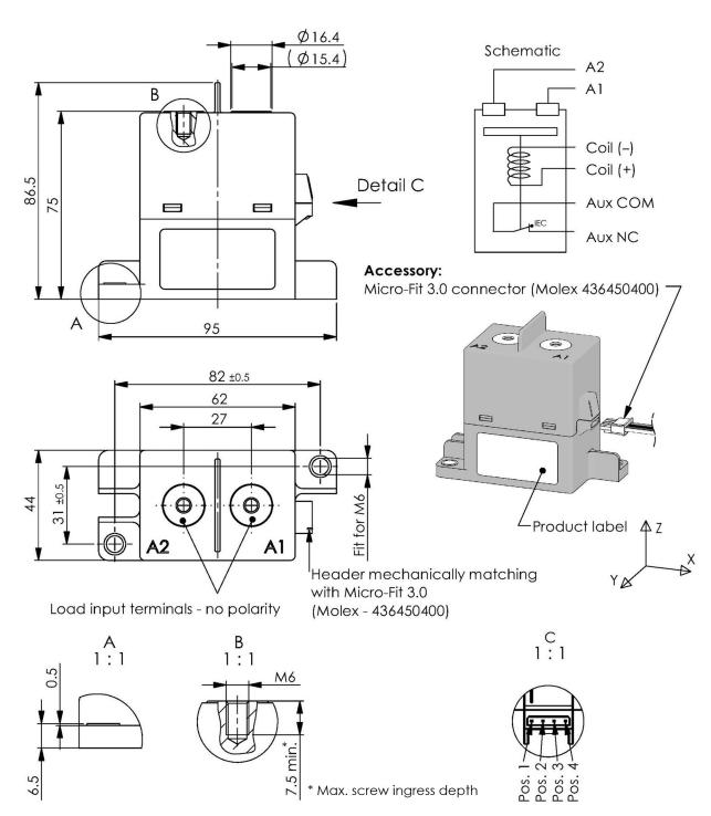
In case of no tolerance shown in dimensional drawing, general tolerances apply: dimension  $\leq$  10 mm;  $\pm$  0.3 mm; dimension 10 to 50 mm;  $\pm$  0.6 mm; dimension > 50 mm;  $\pm$  1 mm
