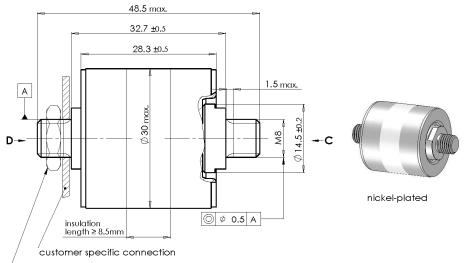
max.torque = 8 Nm counter-hold with 13mm wrench to minimize torque charge
