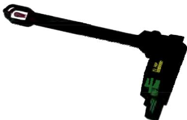
An electronic circuit connected downstream of the sensor signal evaluates the measured temperature on the basis of reference values and supplies a signal that merely switches the compressor of the coolant circuit on or off. This circuit is integrated into the sensor casing or in the case of a cabled sensor placed just behind the actual sensor.
