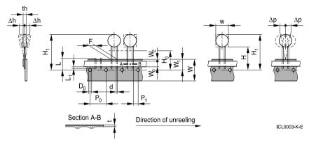
**Lead spacing F = 7.5 mm** (taping based on IEC 60286-2) for the following types: P11, P13, S237, S238 and S364
