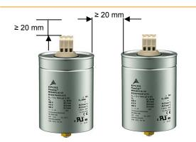
Fig. 3: Minimum distance between PFC capacitors of the PhaseCap series
