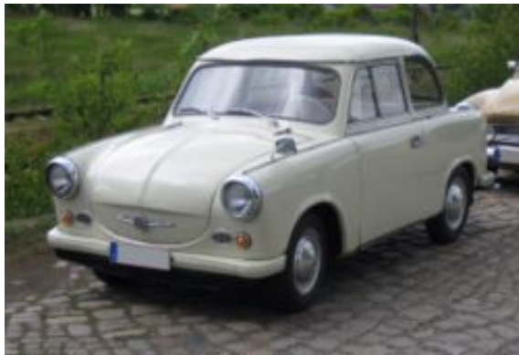
Fig. 1: The Trabant P50, produced in the late 1950s with a plastic shell
