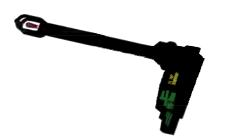
An electronic circuit connected downstream of the sensor signal evaluates the measured temperature on the basis of reference values and supplies a signal that merely switches the compressor of the coolant circuit on or off. This circuit is integrated into the sensor casing or in the case of a cabled sensor placed just behind the actual sensor.
