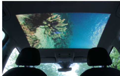
Interior Roof Projection
