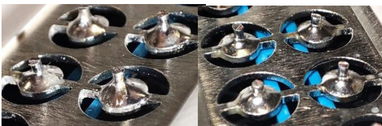
Figure 19. Detailed view of the soldering island after vibration tests
