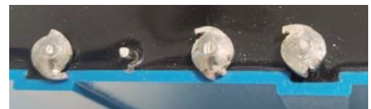
Figure 8. Setup (left) and fracture of the solder islands (right). The capacitors were not glued or fixed to the busbar.
