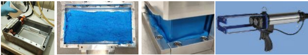
Figure 12. (Left) Manual mixing with supplier Shin-Etsu with gap filler KE1897S A/B. (Center) Supplier B with gap filler B-5 manual mixed. (Right) Recommended pneumatic gun for a proper mix.
