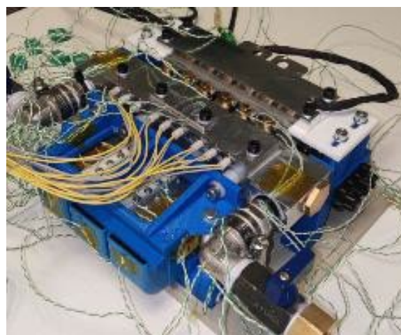
Figure 4. Demonstrator with cooler, water flow and heaters to simulate different scenarios of cooling and different temperatures.
