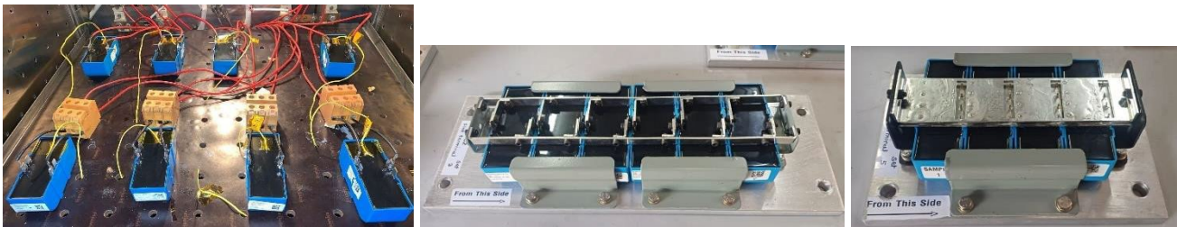
Figure 9(d). xEVCaps during testing: High-temperature operating lifetime (left). Test fixtures for AEC-Q200 vibration test (center and right)
