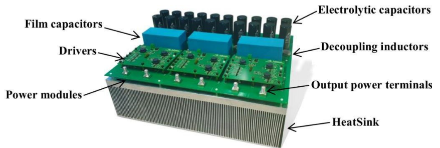
Figure 2. Demonstrator of a 1500 V solar inverter by Infineon. Easy 3B module: 1200V TRENCHSTOP™ IGBT7 + 1200 V CoolSiC™ MOSFET. TDK Electronics: Hybrid DC-link capacitor bank: High-frequency film capacitor (blue) + aluminum electrolytic (black) [2].
