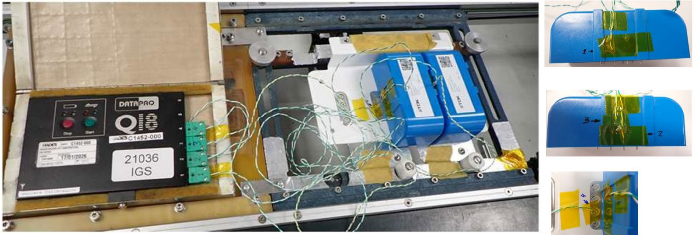
Figure 13. Details of selective wave soldering trials with the datalogger and probe position. Only bottom pre-heating, reaching a temperature of +60 °C on the busbar (bottom) in 75 s.
