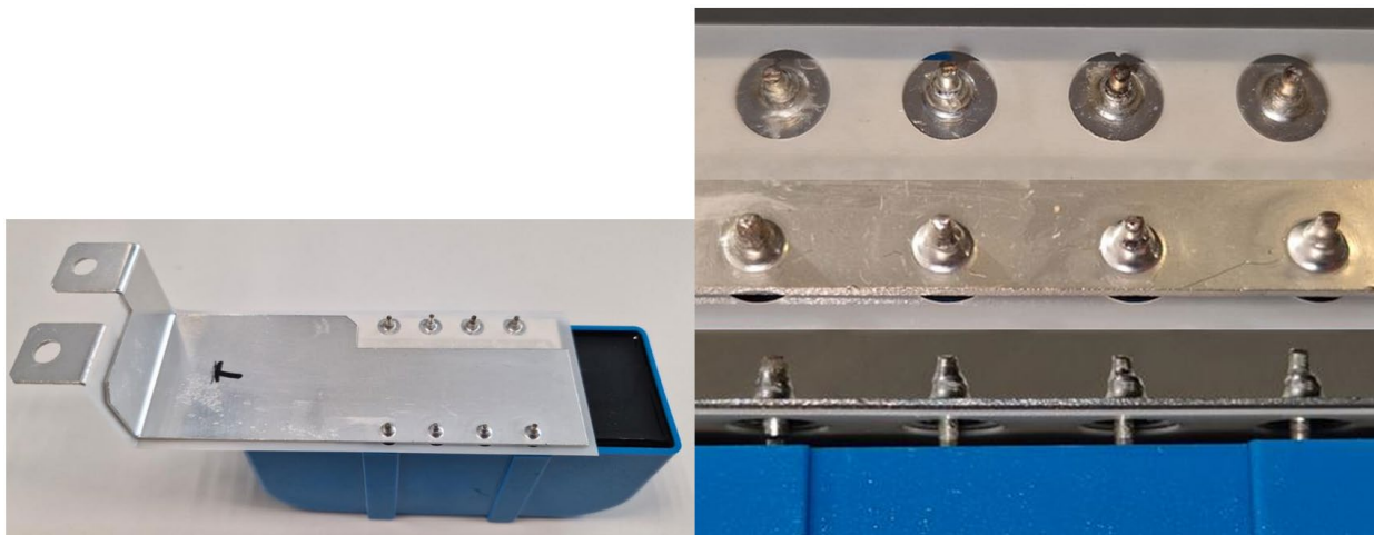
Figure 17: xEVCap with own TDK busbar design. After laboratory trials of the soldering process. Details of terminals and finishes.
