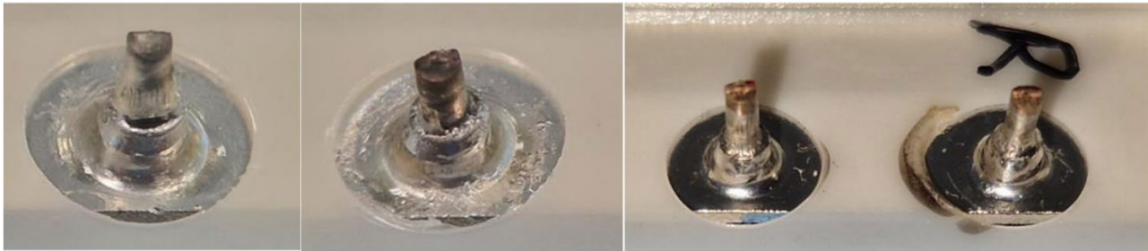
Figure 10: Solder gap (left), burnt tip (center), damaged insulation sheet (right).
