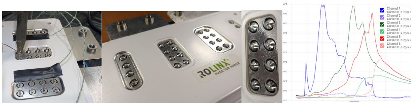
Figure 4: Detail of the manual soldering process and finished soldering points with temperature monitoring: Channel 1: Busbar surface, next to capacitor 1. Channel 2: Capacitor 1. Channel 3: Busbar surface, next to capacitor 2. Channel 4: Capacitor 2. Channel 5: Busbar surface, next to capacitor 3. Channel 6: Capacitor 3. (Rogers Corporation)
