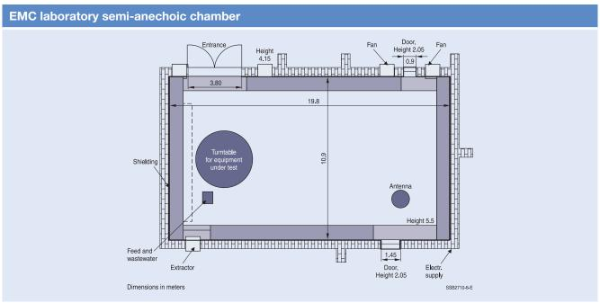
The EMC laboratory features a semi-anechoic chamber for field strength measurements in accordance with the relevant standards at a measurement distance of 10 m between the antenna and the equipment under test.
