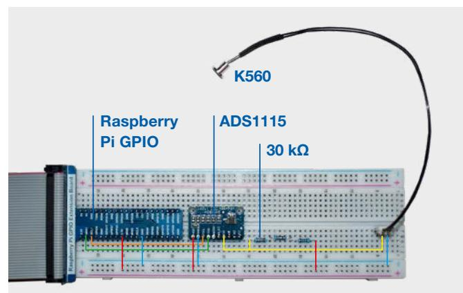
Figure 1: Evaluation circuit and breadboard wiring using a K560 thermistor probe from TDK for surface temperature sensing, an ADS1115 from TI as 16-bit ADC connected to a Raspberry Pi 3 via I<sup>2</sup>C.
