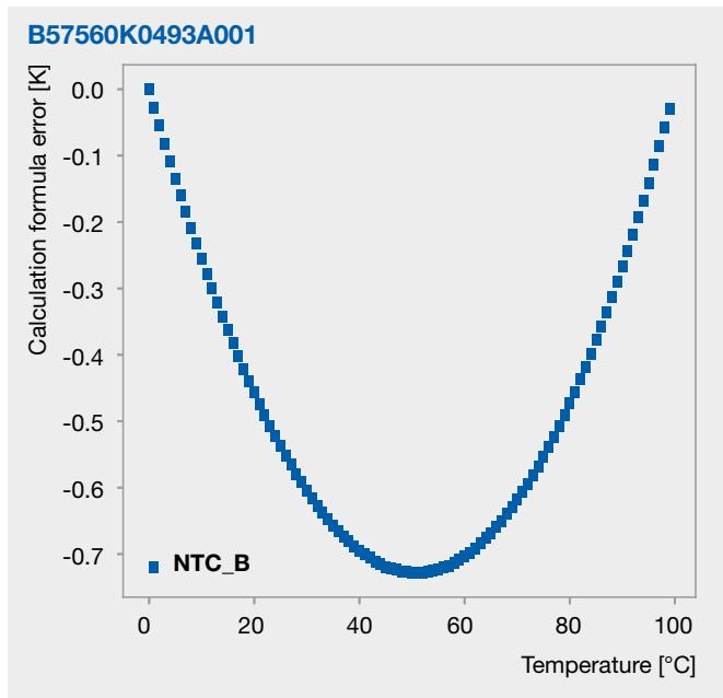
Figure 4: Difference between actual temperature and calculated temperature based on equation (1)
