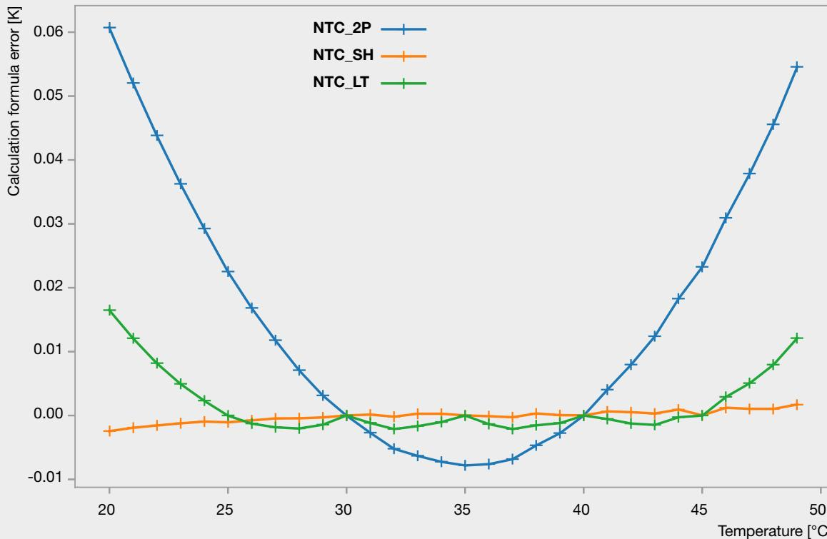
Figure 7: Difference between actual temperature and calculated temperature from the three different algorithms
