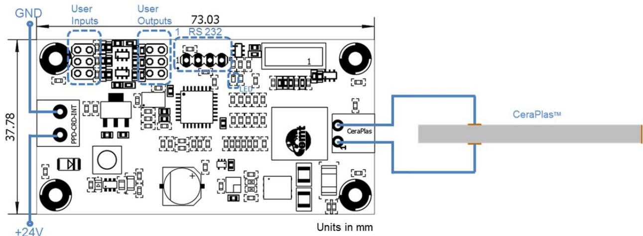
Fig. 1. CeraPlas driving circuit connection setup
