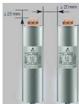
Figure 3: Minimum space over and between the capacitors.
