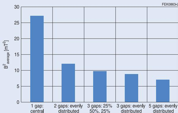
The  $L_{\text{DC}}$  behavior depends on the size and location of each gap size (the total air gap size is the same).
