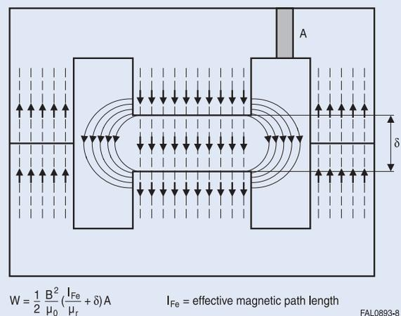
However, the bigger the air gap, the higher is the fringing flux that spreads around it, e.g. into the copper winding. This phenomenon leads to higher losses (e.g. copper losses).
