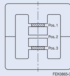
The different air gap structures shown above feature in lower losses from left to right and a correspondingly lower rise in temperature. As a result, the temperature of the core-coil system is lowest for core geometry with 3 evenly spaced gaps. Because the flux density of a ferrite is very temperature-sensitive decreases with increasing temperature, the  $L_{\text{DC}}$  parameter exhibits a visible improvement depending on the number and position of the air gaps.
