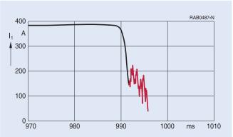
Typical contactor part extinguishes in 4.6 ms with lots of fluctuations, which heats up the main contacts.
