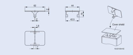
Cover shield to order if required: B88269X2200C101 = 10 pcs. cover shields in a box
