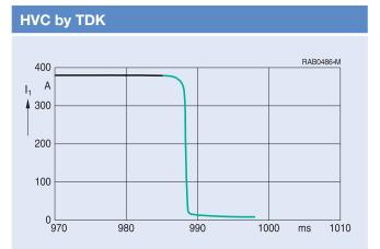
HVC part extinguishes in 1.2 ms with a clear break of current.
