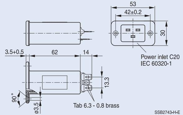
Dimensional drawings of snap-in versions, snapper on vertical side
