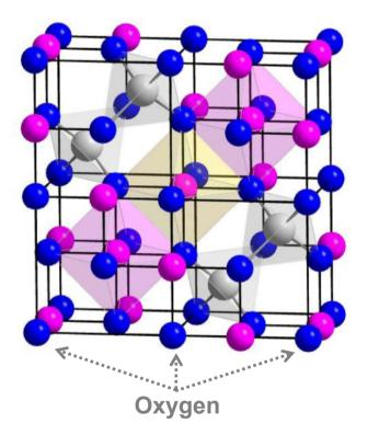
Spinel structure  $NiMn_2O_4$  ( $AB_2O_4$ ) For NTC A places = <u>Ni</u>, (Co, Zn, Al, Fe) – grey B places = <u>Mn</u>, (Ni) - rose
