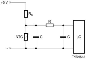
NTC thermistors are a reliable to avoid high thermal stress of LEDs.
