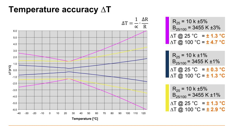
It is important to know the operating temperature range and therefore the tolerance (both R and B value tolerance). With this information the best fitting NTC thermistor can be selected for the application.
