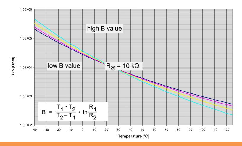
The higher the B value the steeper the curve the larger the resistance change.
