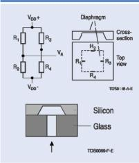
Measurement of pressure with silicon sensor dies is based on the piezo-resistive effect. This is utilized in a silicon diaphragm in which mechanical stress leads to a change of resistivity. The mechanical stress results from a pressure difference across the diaphragm.
