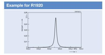
• Center frequency tolerance: down to ±25 kHz
