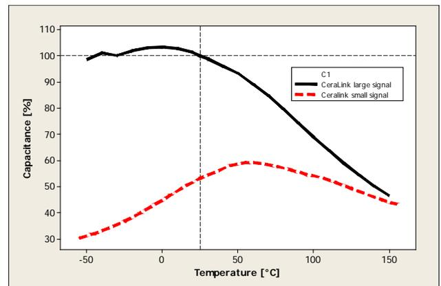
Figure 7 - Capacitance in dependence on temperature ( $V_{DC} = 400 \text{ V}$ )
