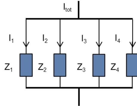
Figure 6 - Simple parallel connection of impedances
