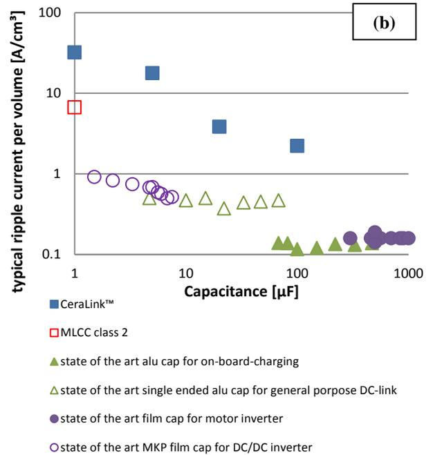
**Figure 3 - comparison on capacitance per volume (a) and current per capacitor volume (b), please note, that the figures only account for capacitors with same voltage rating**
