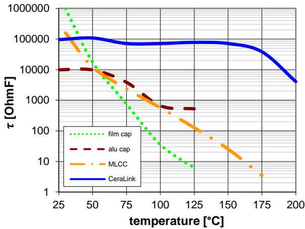
Figure 4 - insulation properties over temperature, capacitors with same voltage rating
