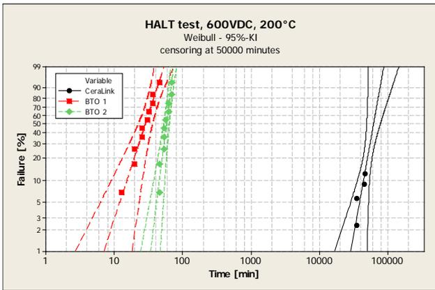
Figure 5 - lifetime at high temperatures
