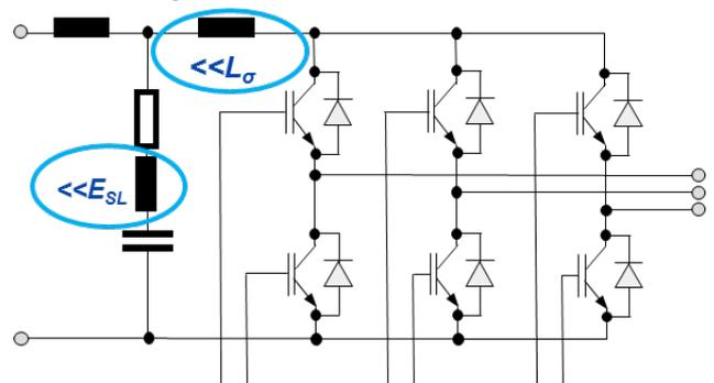
**Figure 8 - commutation loop inductance with ideal semiconductors in a 3 phase configuration**
