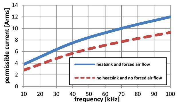
**Figure 2 - typical permissible current depending on the cooling condition (ambient temperature 85 °C, measurement of 1 µF 500 V device), the permissible current corresponds to a device temperature of 125 °C**
