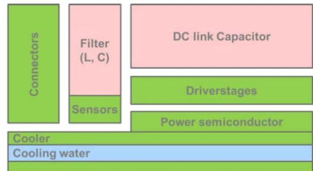
**Figure 1 - principle block picture and size comparison of a motor inverter (source: Volkswagen AG [3])**
